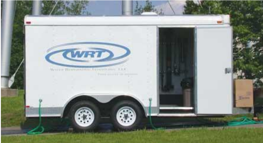
Water Remediation Technology offers a pilot testing system enclosed in a trailer. The modular pilot system can also be mounted inside a treatment facility.
